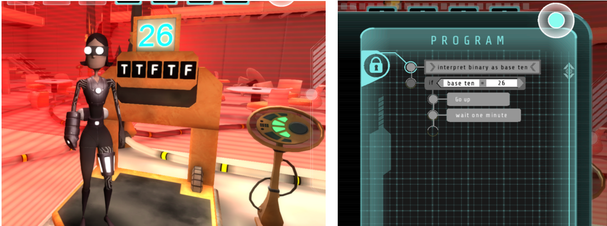
Figure 3.2. Binary challenge. (Left) a binary lock device that students must unlock. The T (true) tiles indicate the bits are 1, whereas F (false) tiles denote 0. The current binary number is 11010 and the corresponding base-ten number, 26, is displayed on the device as immediate feedback. (Right) the visual programming interface displaying the binary lock's program.
